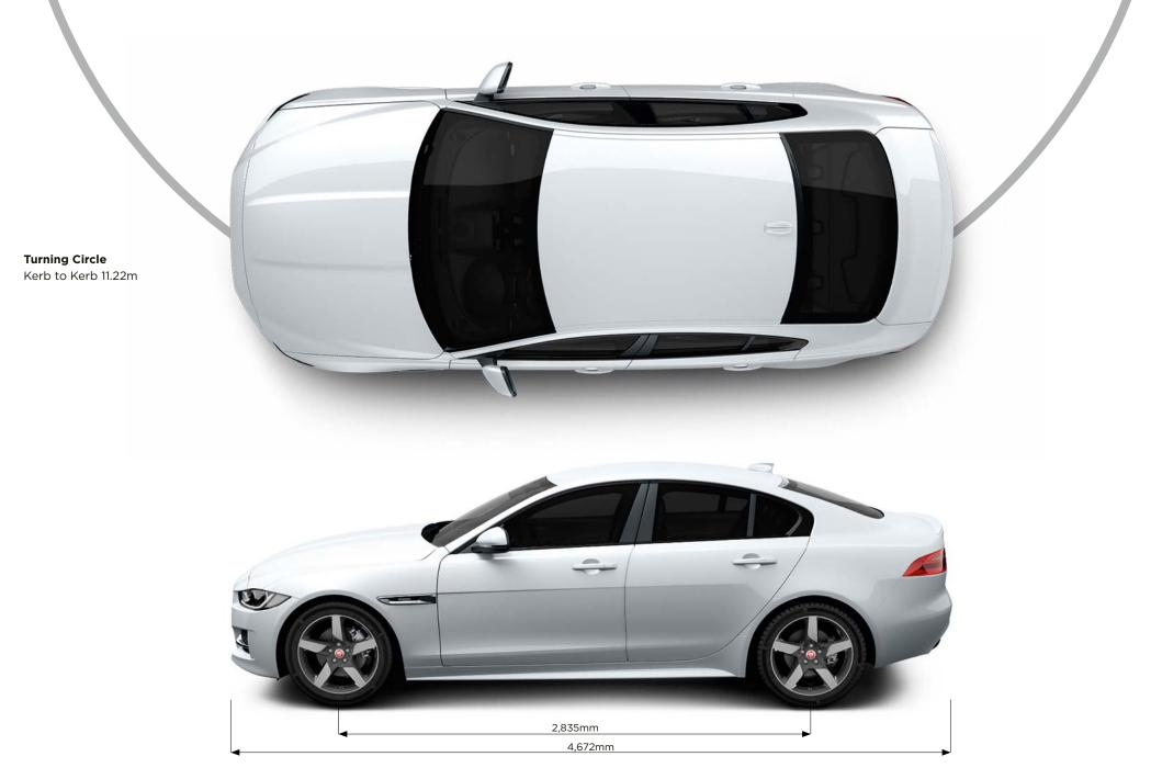
Dimensions were measured with vehicle at unladen weight. (measured by VDA standard test method using 200 x 100 x 50mm blocks.) VEHICLE SHOWN: XE R-SPORT IN YULONG WHITE WITH OPTIONAL FEATURES FITTED (MARKET DEPENDENT)
